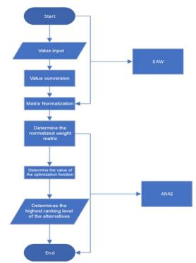
Figure 1. Flowchart of the Merger of SAW and ARAS
