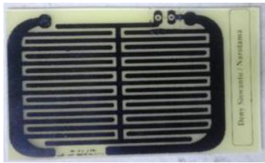
Sumber: Siswanto & Winardi (2015) Gambar 4b. Penampang sensor air
