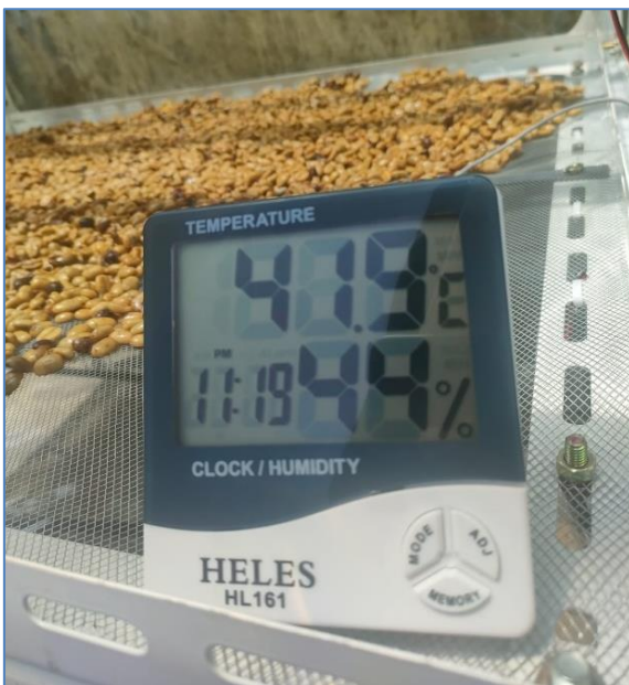
Source: (Research Results, 2024) Figure 8. Initial Temperature and Humidity of Coffee Beans Entered
