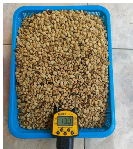
Source: (Research Results, 2024) Figure 10. Results of Automatic Drying of Arabica Coffee Beans
