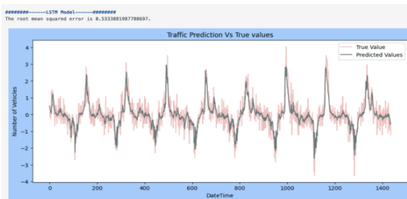
Source: (Research Results, 2025) Graph of Comparison of Predictions and Actual Values on Road 2 Using the LSTM Model with Adam Optimizers
