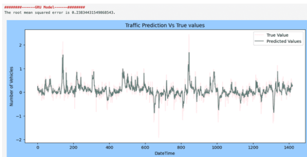
Source: (Research Results, 2025) Figure 13. Graph of Comparison of Predicted and Actual Values on Road 1 Using the GRU Model with Adam Optimizers
