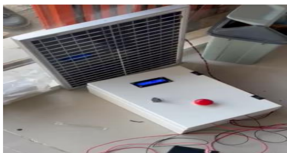
Figure 5. Solar panel and component box configuration.
