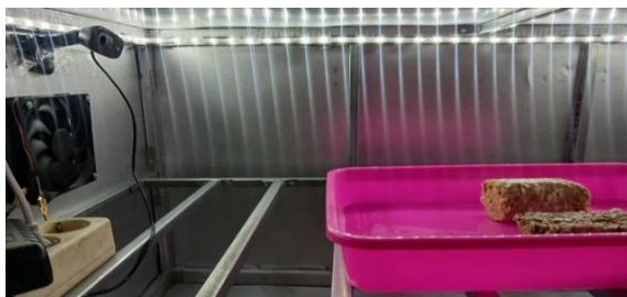
Figure 3. The actual condition of the fermentation box, LED illumination, and camera position during image acquisition
