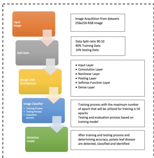
Source : (Research Results, 2023) Figure 1. General Scheme for Image Classification
