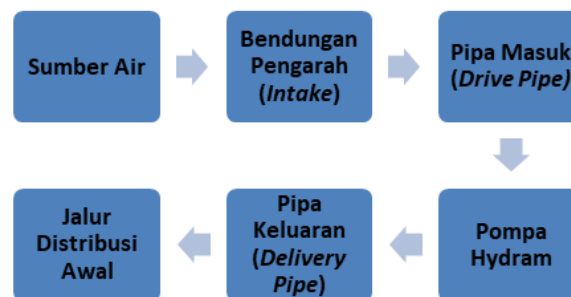
Gambar 2. Alur Sistem Pompa Hydram
