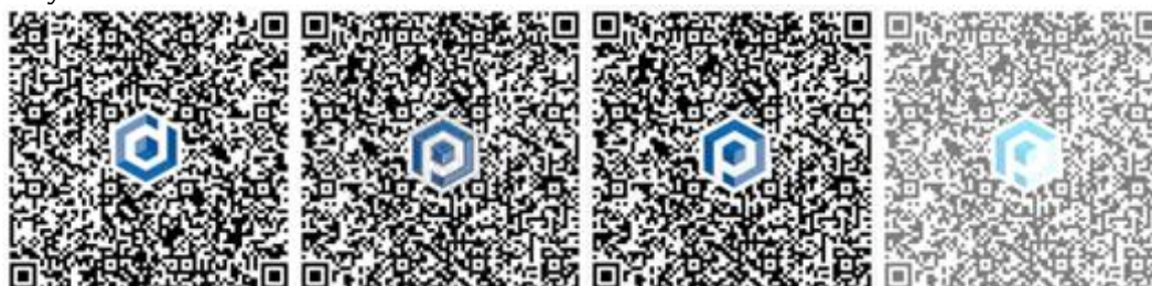
Figure 6. QR Code Robustness Testing Under Image Distortions (Rotate, Sharpen, Poisson, Gaussian)
